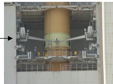
Vehicle support structure (Move away upward at liftoff)
