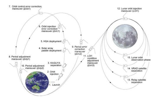
\* Period adjustment maneuver( $\Delta Vp1$ ): orbit control to adjust the KAGUYA's orbit period (8 in the above figure) \* Period error correction maneuver( $\Delta Vc2$ ): orbit control to correct errors with  $\Delta Vp1$  orbit control and determination (9 in the above figure)
