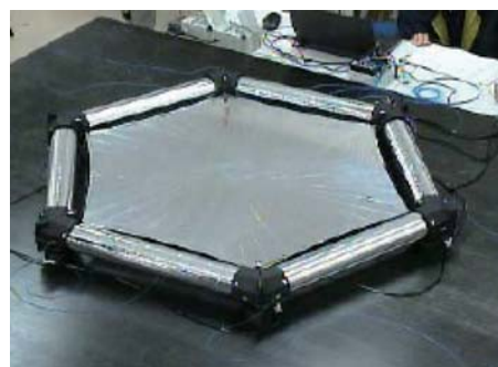
Fig. 4 Test-fabricated inflatable structure
