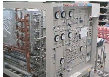
Valve reliability evaluation test facilities
