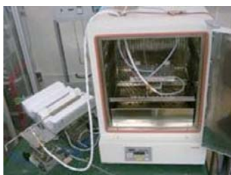
Fig. 3 Sabatier reactor and oxygen reproduction equipment using water electrolysis
