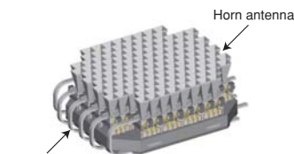
APAA installed on WINDS
