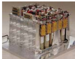
Lithium-ion battery assembly
