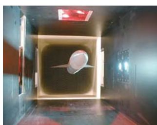
Fig. 1 (a) AGARD-B model. The forces acting on the model were measured by one of the largest magnetic support systems in the world
