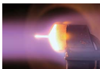
Fig. 4 Graphite heating test in an induction-coupled plasma heated wind tunnel.
