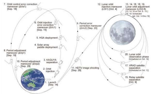
\* Lunar orbit adjustment maneuver (LOI4): orbit control to lower the KAGUYA's altitude in the injected lunar orbit (16 in the above figure)
