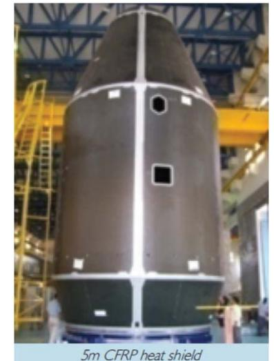
5m CFRP heat shield
