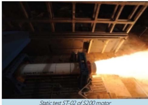
Static test ST-02 of S200 motor
