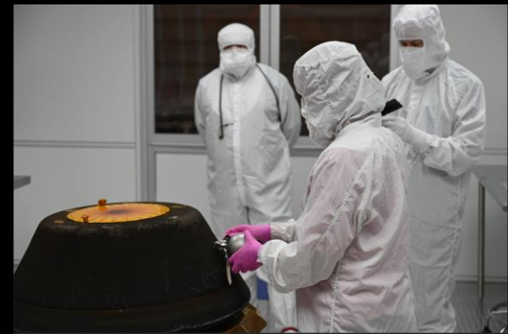
Initial Disassembly of Sample Return Capsule and Connection of Nitrogen Flow to Sample Canister in Temporary Cleanroom in Utah on Landing Day: September 24, 2023
