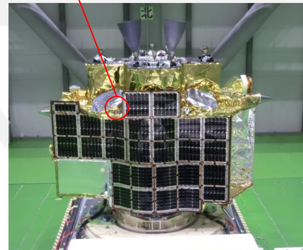
LRA(Laser Retroreflector Array) provided by NASA. The LRA consists of an array of multiple mirrors that are retroreflective and reflect light back in the direction of origin. Mass is approximately 21g.
